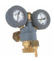
Mini pressure regulator with flow gauge, i.e. with indication I/min on secondary gauge. Integral safety valve. The flow is adjusted on the regulating screw by changing the secondary pressure and through a throttle valve in the outlet.
