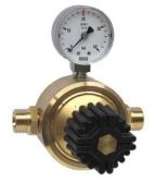
Low pressure regulator with mounted working pressure gauge and regulating screw for the adjustment of the working pressure. Diaphragm made of NBR, filter in the inlet made of sinter bronze.
