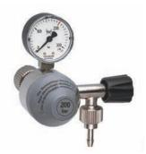
Pressure regulator with contents gauge for indication of cylinder pressure, but without working pressure gauge; with preset working pressure and integral safety valve. A fine regulation spindle enables a precise regulation of small quantities of gas (also for the aeration of aquariums).
