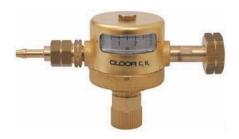
Pressure regulator with working pressure gauge, compact and robust construction. Suitable for applications where propane and oxygen are used in combination. Material of diaphragm an valve seat is NBR.
