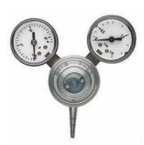
Pressure regulator with cylinder contents gauge. Flow rate with fully opened pressure adjusting screw alternatively 0.25, 0.5, 1.5 or 2.5 l/min. The pressure adjusting screw serves also as a shut-off valve. Particularly suitable for applications in which a precisely defined flow rate and secondary pressure are required.
