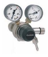
Pressure regulator with pressure and contents gauges, integral safety valve and shut-off valve in the outlet. Inlet at the rear, pressure adjusting screw at the front. Material: brass, nickel plated. Sintered filter in bronze, diaphragm made of Neoprene EFFBE.
