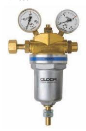
With working pressure and contents gauges and integral safety valve. With pipeaway facility fitted to safety valve for venting gases to atmosphere. Standard version with working pressure up to 10 bar. Also available with working pressure up to 20 or 30 bar (see below).
