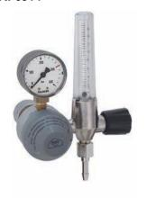
Pressure regulator with fitted flowmeter with fine regulation spindle (serves at the same time as shut-off valve) and safety valve. Accuracy of measurement of flowmeter +/-10%. Available for three different flow rates (see below).
