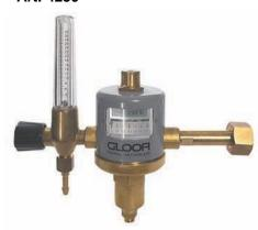
With fitted flowmeter and gauge showing cylinder contents. Integral safety valve and shut-off valve on flowmeter. Accuracy of measurement of flowmeter +/-10%. Available in three different flow rates (see below).
