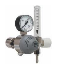
Pressure regulator with contents gauge and fitted flowmeter; integral safety valve. The flowmeter design ensures a clear reading of the delivered flow rate. Diaphragm made of Neoprene EFFBE; also available with Teflon coated diaphragm upon request.
