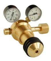
The pressure regulator is available in version for working pressure up to 100 bar or up to 200 bar. The working pressure is infinitely adjustable on the handwheel between 10-100 bar, resp. between 10-200 bar. For an easy pressure adjustment the handwheel shows at the front a hexagon, so that the pressure adjustment can also be made by means of a socket wrench 8 mm.
