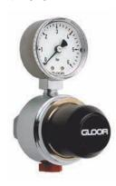
Low pressure regulator for high purity gases (6.0). Sintered filter in inlet. Pressure regulation through metal diaphragm. Working pressure fully variable as required from 0–4 or 0–10 bar.
