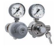
Two-stage pressure regulator with indication of cylinder content and working pressure. Particularly suitable for applications requiring a very constant secondary pressure. Working pressure preset from 0.5 to 3 bar (as required). Also available with Teflon coated diaphragm for analysis equipment.
