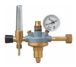
Pressure regulator with contents gauge and with built-on flowmeter. Integral safety valve and shut-off valve on flowmeter. The flowmeter design ensures a clear reading of the delivered flow rate. Accuracy of measurement of the flowmeter +/-10%. Available in three flow rates (see below).
